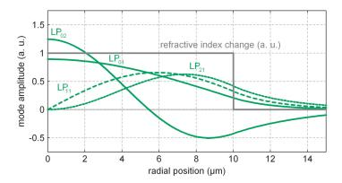
For example,  $LP_{02}$  means that l=0 (i.e., there is no  $\phi$  dependence) and m=2. The fundamental mode  $LP_{01}$  is closest to a simple Gaussian profile, extending somewhat beyond the core.
