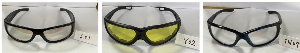
Fig. 10 Three pairs of goggles that had satisfactorily passed the Z87.1 test.
