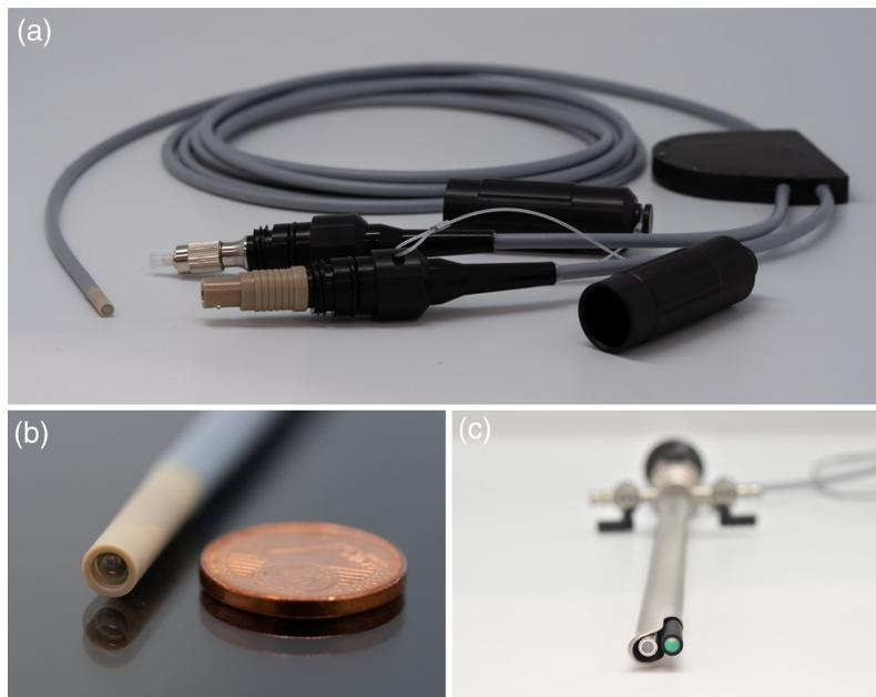
**Fig. 7** Photographs of completely encapsulated OCT/A probes, showing the proximal (a) end connectors, (b) the scale of the 4.5-mm distal end, and (c) the probe introduced into a commercial cystoscope.
