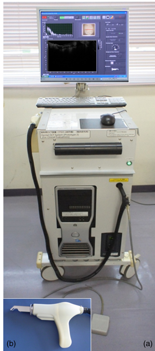
Fig. 1 The swept source optical coherence tomography (SS-OCT) system used in this study. (a) An overview of the SS-OCT machine including screen, interferometer, scanning laser source, and data processing PC. (b) A hand-held probe of the SS-OCT.
