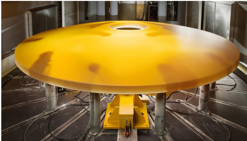
Fig. 24 ESO ELT ZERODUR® secondary mirror blank with 4.25-m diameter, 100-mm thickness, and extreme convex curvature as delivered from Schott in January 2019.
