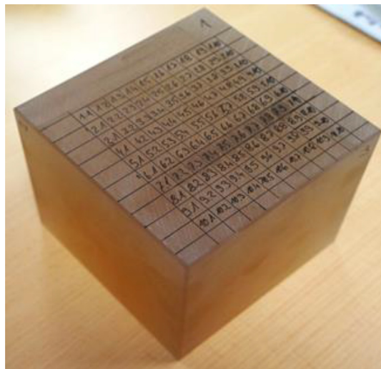
Fig. 8 ZERODUR cube 100 x 100 x 100 mm 3 cut in 100 samples. 13
