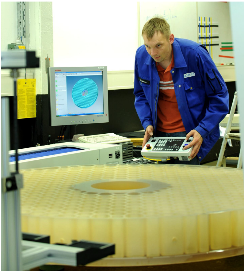
Fig. 21 Solar telescope GREGOR 1.5-m diameter \times 161-mm-thick primary mirror, 420 pockets 8-mm rib thickness, and 65% weight reduction.
