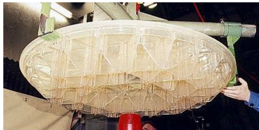
Fig. 20 GEMINI telescope 1-m secondary mirror with 4-mm rib thickness 45 kg 85% weight reduction.
