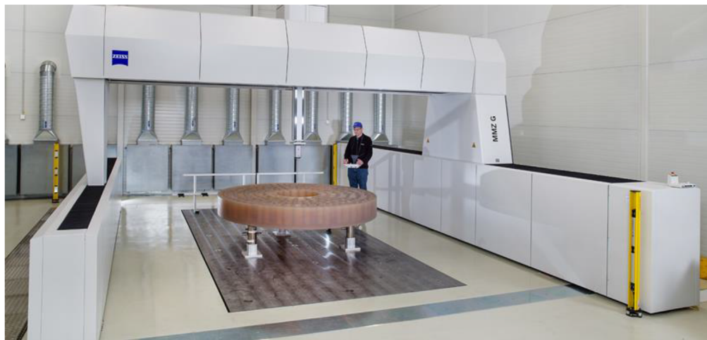
Fig. 25 Schott's new 5-m coordinate measuring machine with ZERODUR® lightweight mirror blank. Maximum measurable dimensions are 5 m × 6 m × 2 m. Temperature stability: better than 0.3 K per day. Maximum deviation found during calibration 2 μm at 2.5 m radius.
