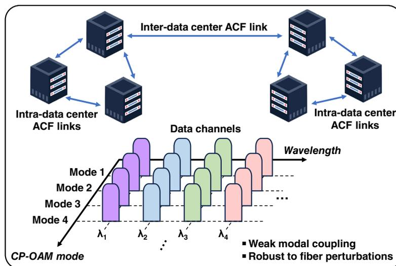
**Fig. 1** The paper by Wang et al. provides valuable insights on how to efficiently add mode multiplexing for cost-effective and high-capacity fiber links. One potentially impactful application could be in significantly increasing the data capacity of future intra- and inter-data center links by adding mode multiplexing using CP-OAM modes in ACFs, which is compatible with WDM.
