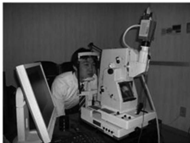
**Fig. 4** A photo showing the outlook of the prototype. We applied a polarization analysis camera instead of the usual CCD camera of the fundus camera. A 1/4 wave plate and a polarization filter were also placed in the illuminating path for circularly polarized light illumination.
