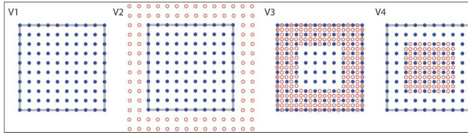
**Fig. 2** Source grid arrangements applied in the phantom studies. The defined RoI is marked by a gray square and the blue dots indicate the commonly utilized sources (see V1). V2 shows the measurement series, where additional source positions (red circles) have been placed outside the RoI. V3 and V4 demonstrate the refinement of sources (red circles) that have been embedded in the outer and inner grid. (Color online only.)
