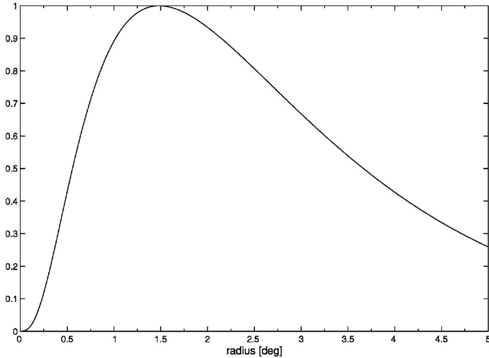
**Fig. 6** Change of the strength of the Henle fiber birefringence signal as a function of the distance from the foveal center as measured in the plane of the photodetector (1 deg of visual angle=1.96 mm at the photodetector).
