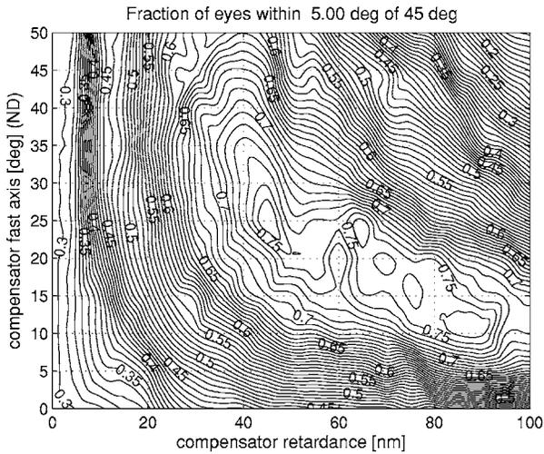
**Fig. 11** Calculating an optimal fixed corneal compensator: fraction of eyes (RE+LE) falling within  $\pm 5$  deg of 45 deg bow-tie orientation, as a function of compensator retardance and fast axis azimuth.
