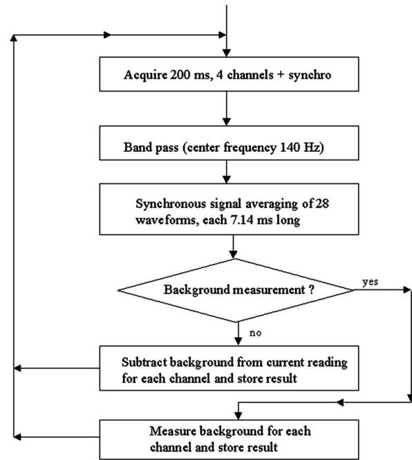
**Fig. 4** Digital signal processing algorithm (simplified).
