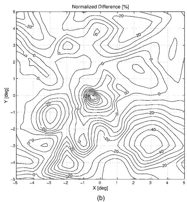
**Fig. 7** Result of the model for the normalized difference ND as a function of the distance between foveal origin and the center of the four-quadrant photodetector. The distance is in degrees of visual angle.
