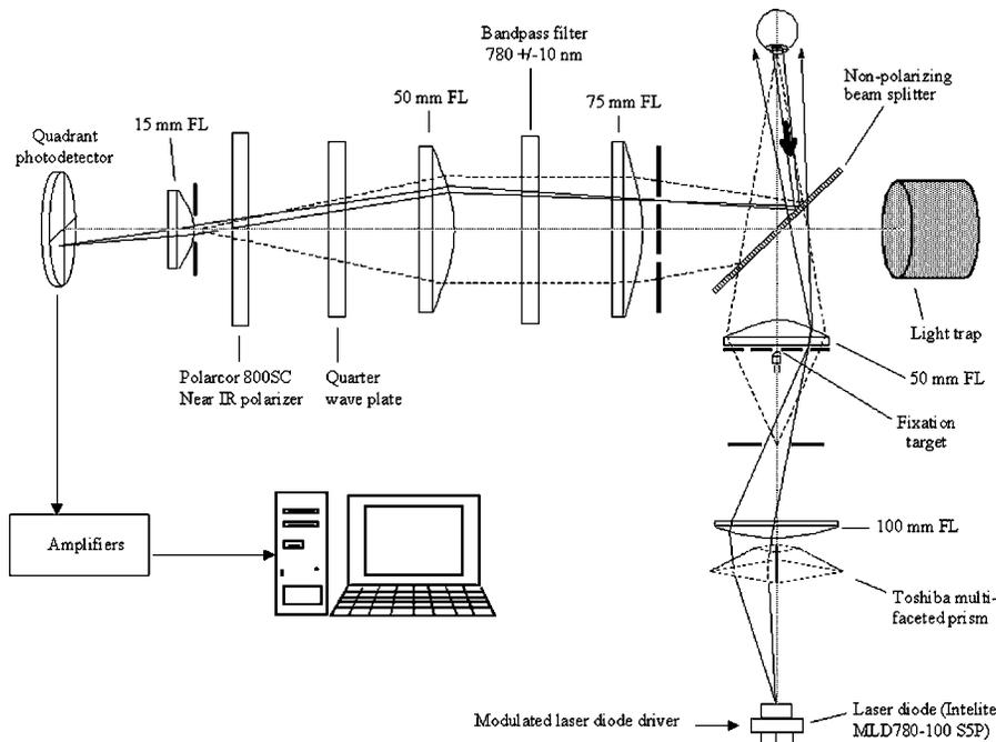
**Fig. 2** Instrument design, showing the illumination and detection light paths for one of the four spots of light, not to scale.
