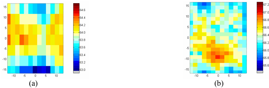
Figure 4: reticle CD fingerprint for three DPL reticle sets, measured with reticle CD SEM (nm CD@1X) (a) 3\sigma=0.9\text{nm} , and (b) 3\sigma=0.6\text{nm} [9,10] (a) was used for LELE results in this paper. (b) was used to gather experimental results for spacer process.
