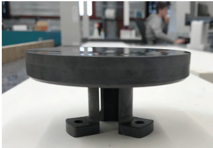
Figure 8. SiC mirror optimized and realized by MERSEN BOOSTEC and coated with CVD SiC.
