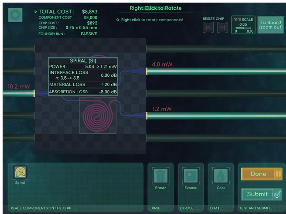
Figure 4. The player has tested the circuit with methane present. They hover over a spiral waveguide, which shows details about light loss due to interface loss (none), material loss (-1.2 dB), and absorption loss (-5 dB).
