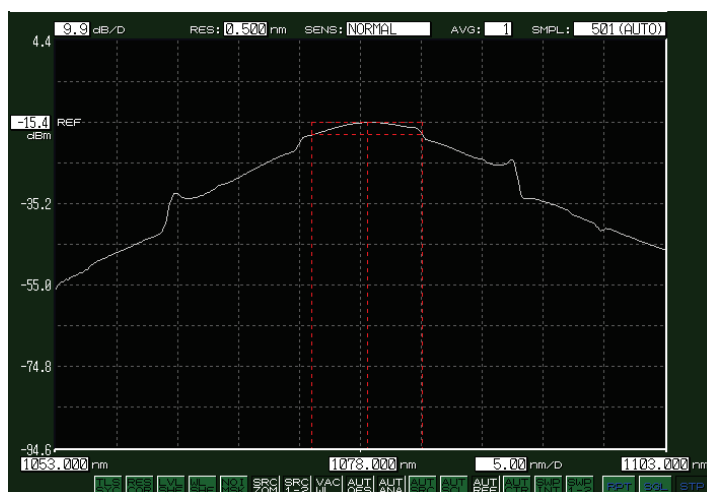
Figure 5. Spectrum of the operating laser, showing a centre wavelength of 1078 nm and a bandwidth of 9.1 nm.
