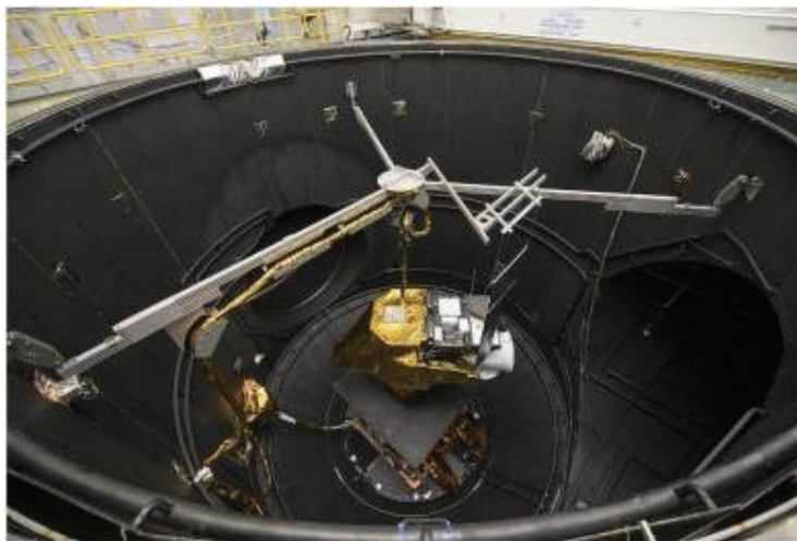
Figure 16: FCI STM entering the ESTEC Large Space Simulator
