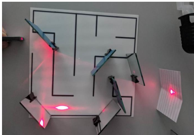
Figure 1. The laser maze demonstration is simple but drives home the law of reflection for students.
