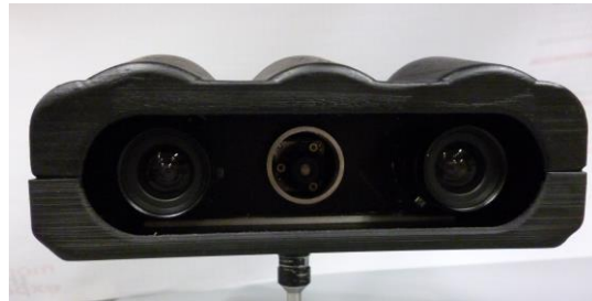
Figure 7: Stereo system with laser projector
