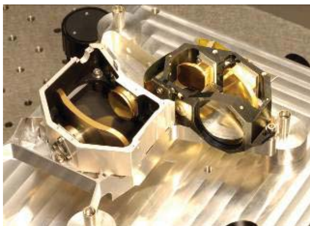
Figure 13: Assembled MERTIS Spectrometer Optics
