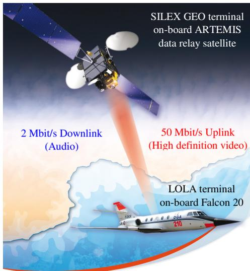
Fig. 1: The LOLA bi-directional optical data link between an aircraft and the Artemis GEO Relay satellite
