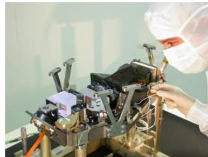
Fig. 4: SiC focal plane prior to integration
