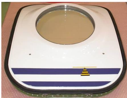
Fig. 12: The optical window mounted on an emergency door of the aircraft
