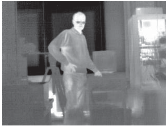
Fig. 11: Infrared image obtained with a 320 x 240 microbolometer FPA
