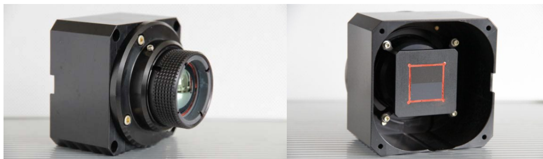
Fig. 4. Optical system breadboard, showing the lenses (left), the filters set (right) and the mechanical support.
