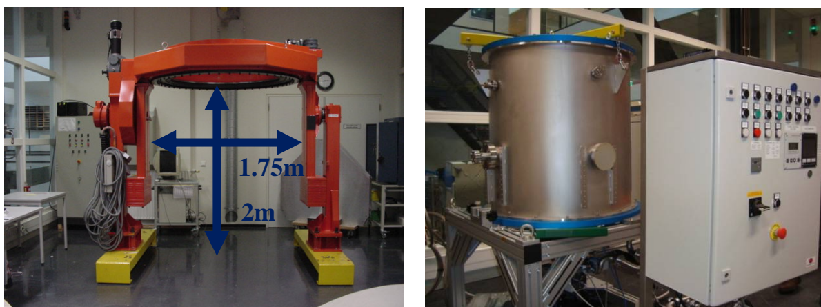
Fig. 4. Left: Telescope movement simulator, capable to position a large cryostat in any orientation with respect to gravity. Right: Large test cryostat with vacuum and cryogenic equipment.
