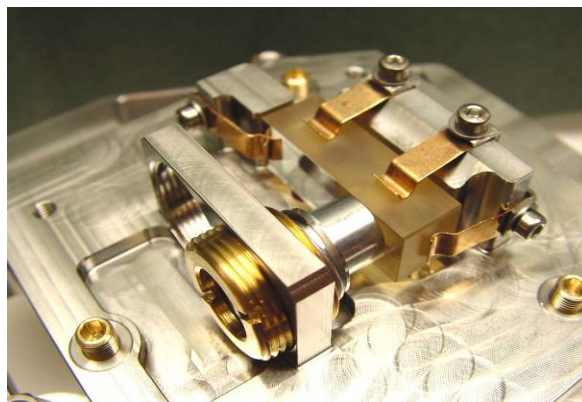
Fig. 8. Cryogenic vacuum CTE measurement setup
