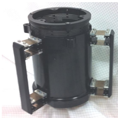
Fig. 4. Frictionless uni-axial linear scanner
