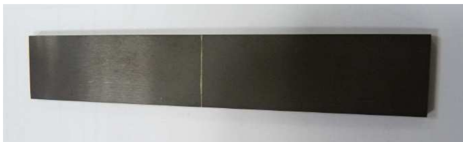
Fig. 6. Silicon nitride sample with a brazed junction at the middle of the sample, for 4-point bending tests
