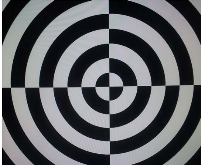
Fig. 5. Image impressed onto the liquid crystal SLM adopted for the development of the prototype.
