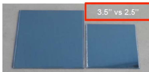
Fig. 9: Sofradir HgCdTe epilayer deposited by LPE on Sofradir substrates
