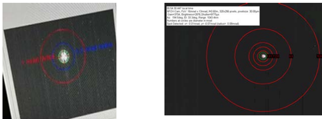
Fig 7. Tracking camera images of TOGS (left) and OGS-OP (right) after link acquisition and engagement of closed optical tracking loops. (Image source: DLR)
