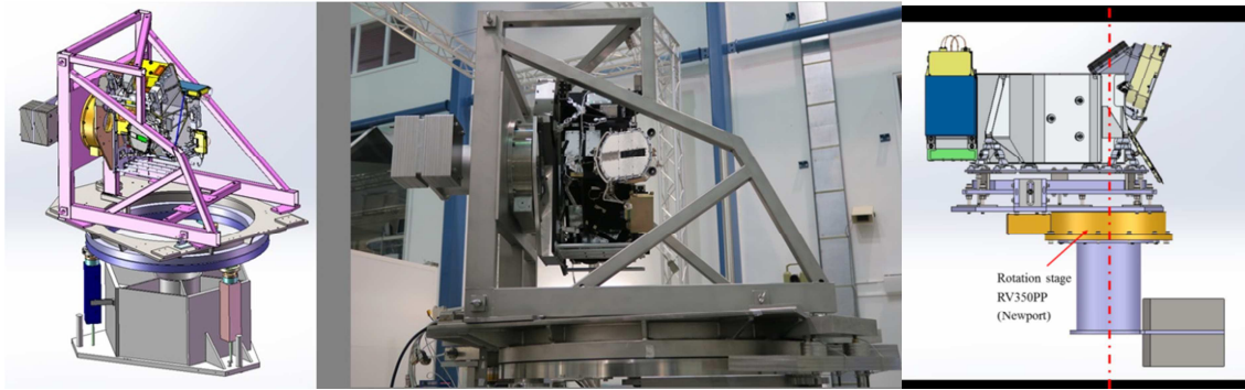
Figure 6: (left and middle) FUV-Instrument mounted on the GSE manipulator. (right) device to allow turret motion compensation.
