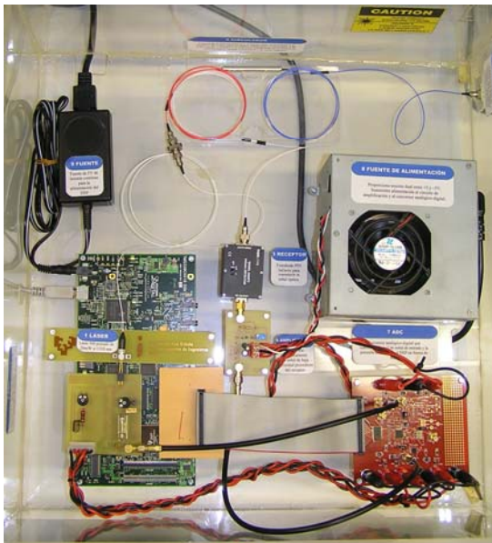
(b) Photograph of the components (interspersed with several power supply units) that constitute the prototype.
