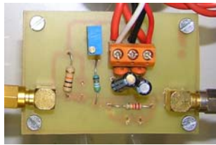
(b) Photograph of the signal conditioning circuit (the amplifier is placed on the back).
