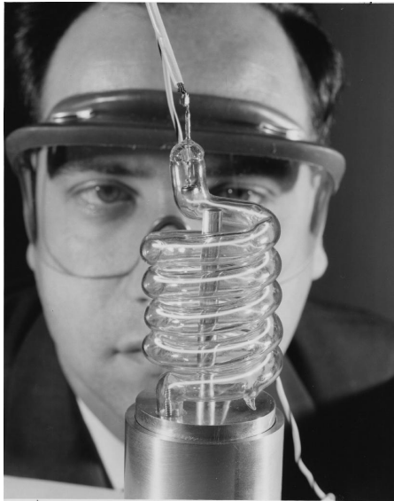
Figure 1: Hughes press release photo showing Maiman behind a larger flashlamp than he used.
