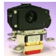
Laser chopper mechanism (ALADIN programme)
