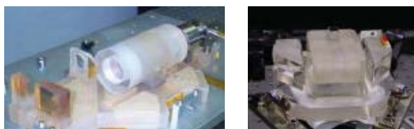
Mie spectrometer based on Fizeau design (left) and Rayleigh spectrometer based on double-edge (right)
