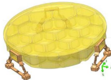
Fig. 4. Illustration of the M1 mirror with MFD (THALES-SESO)
