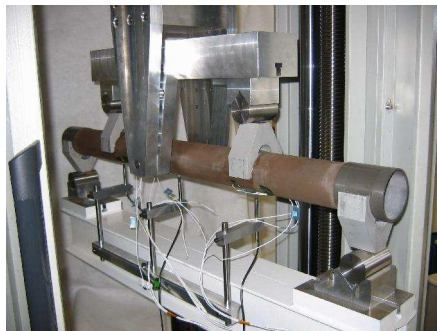
Fig. 1. Test of the first beam in silicon nitride (evaluation phase)
