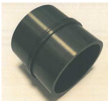
Fig. 7. Ceramic rings after brazing
