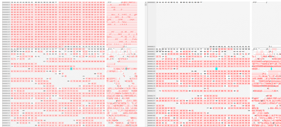
Figure 6. Differences in file header data between the taken image in the No. 1 cell phone and the image downloaded from the computer version of the WeChat.
