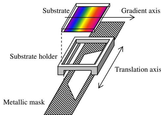
**Fig. 2.** Principle of the masking mechanism
