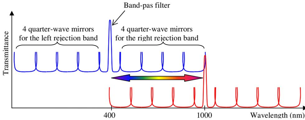
**Fig. 1.** Schematic spectral profile of the coating split in its elementary stacks
