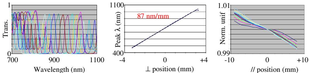
**Fig. 3.** Transmission profiles measured on the band pass variable coating (left), measured thickness gradient (middle), and normalized uniformity measured perpendicularly to the gradient (right)
