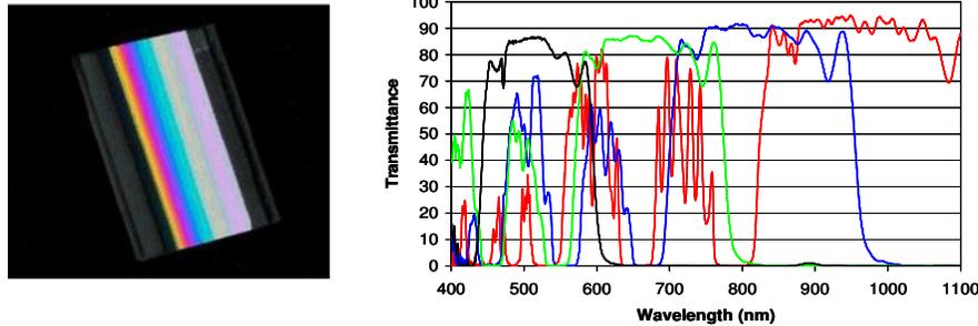
**Fig. 4.** Four measured transmittance profiles across the short-wavelength pass blocking filter with cut off wavelengths at 600 nm (black), 775 nm (green), 950 nm (blue), 1150 nm (red)
