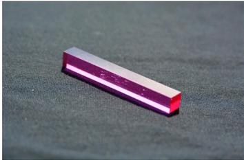
Figure 7 Ruby sample used by Giuliano to characterize laser damage tracks; 6mm x 6mm x 50mm
