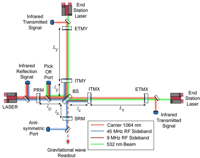
Figure 3. Simplified optical layout. See text for details.
