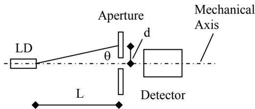
Fig. 1. Measurement setup,  $\theta$ : pointing angle.
