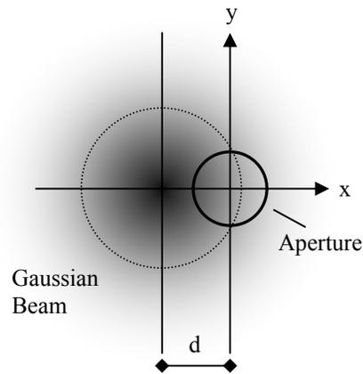
Fig. 2. Positions of laser beam and aperture on aperture plane.
