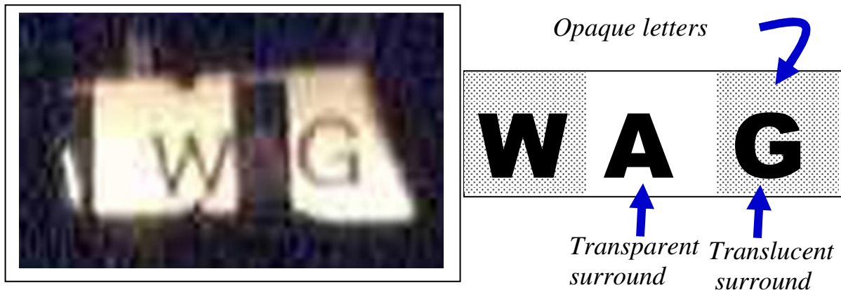
Fig 2. Photograph of the back-lighted translucent-transparent object shown on right.
