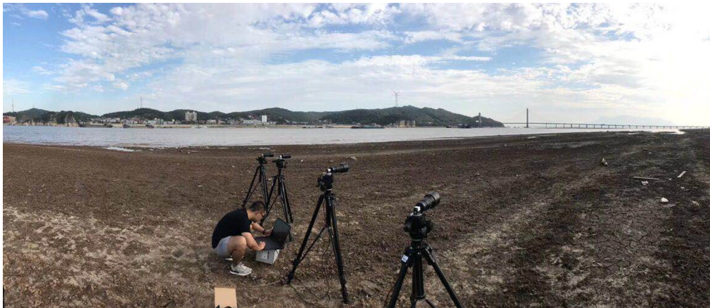
Fig. 8 Deflection measurement of long-span bridge using multicamera 2D measuring systems.
