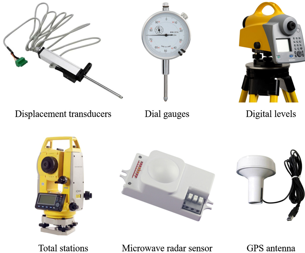
Fig. 1 Several commonly used bridge deflection measurement equipment.
