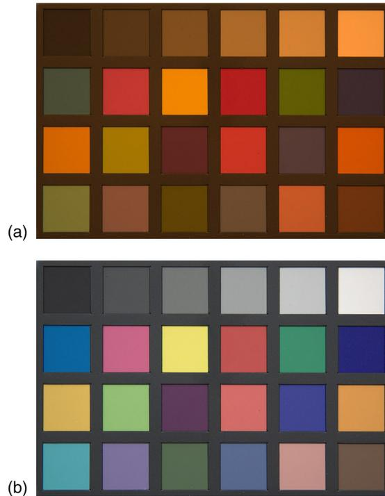
**Fig. 7** (a) Photo of a color chart taken under 2700 K CCT tungsten illumination and converted to the sRGB color space for display without any chromatic adaptation. (b) White balanced photo obtained by including a CAT to adapt the scene illumination WP to the D65 reference white of the sRGB color space.
