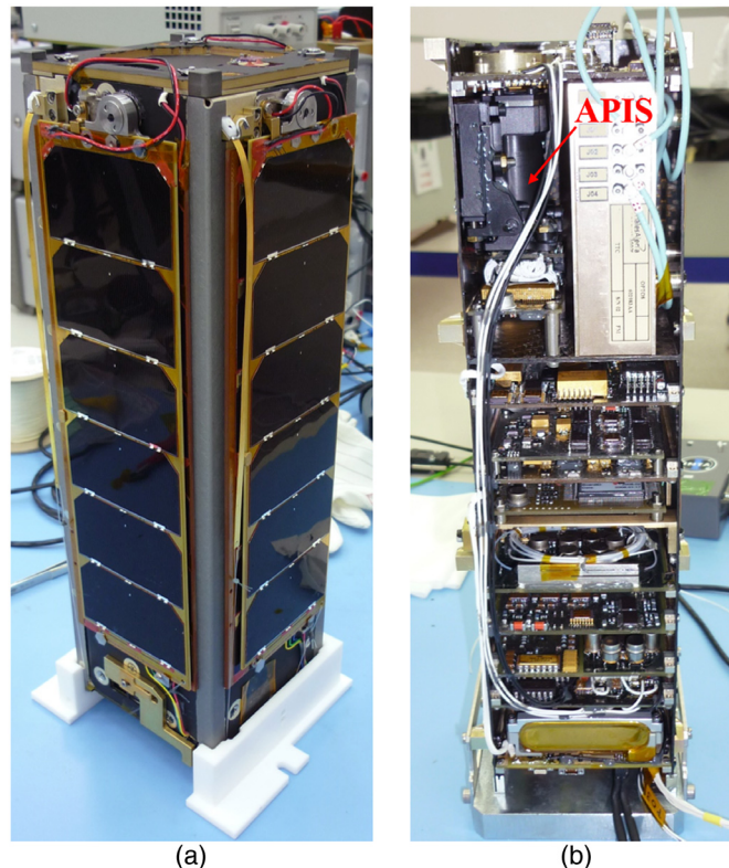
Fig. 1 (a) OPTOS satellite in launch configuration with the panels folded and (b) OPTOS internal structure with APIS assembled in the upper left part.
