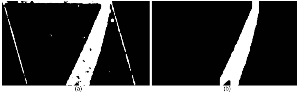
Fig. 5 (a) Mask after threshold is applied to an entropy mask. (b) Mask in (a) processed using binary morphology to remove unwanted artifacts and leave only the contact lens visible.
