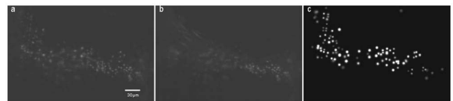
Fig. 4 Particle image processing. (a) Defocusing images acquired in experiments. (b) Background due to microspheres trapped by surrounding tissues. (c) Processed images after background removal, low-pass filtering, particle detection, 2-D Gaussian model, and noise removal.
