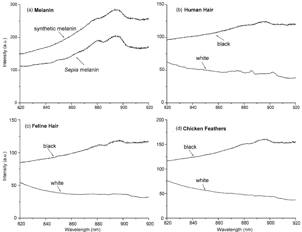
**Fig. 1** NIR autofluorescence spectra (820 to 920 nm) obtained from: (a) *Sepia* and synthetic DOPA melanin; (b) human hair; (c) feline fur; and (d) chicken feathers. Excitation wavelength 785 nm; light intensity 170 mW; and integration time 1 s.
