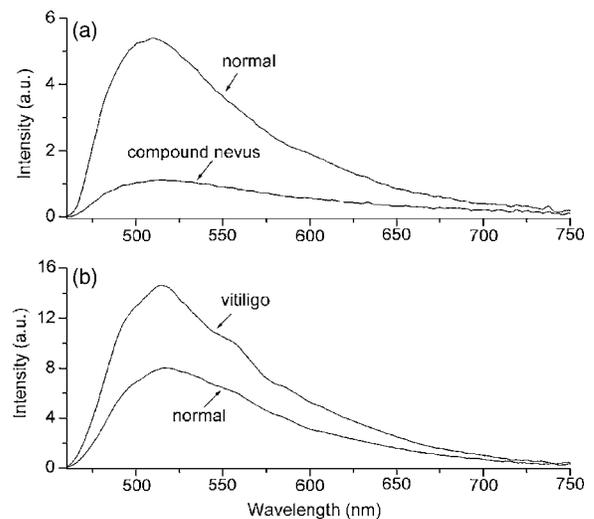
**Fig. 3** Paired autofluorescence spectra in the visible range (460 to 750 nm) obtained from skin lesions and their normal surrounding skin site: (a) compound melanocytic nevus, and (b) vitiligo. Excitation wavelength 437 nm  $\pm$  10 nm; light intensity 9.5 mW; and integration time 0.1 s.
