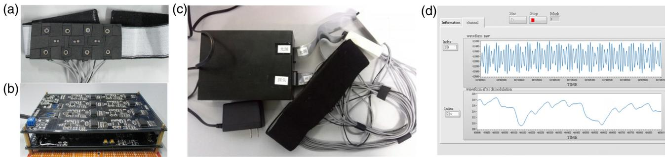
**Fig. 3** The display of the multichanneled fNIRS system. (a) The wearable headset, (b) the disassembled prototype of the hardware motherboard, (c) the device appearance with the size of 125 mm × 110 mm × 50 mm, and (d) the software interface developed based on Labview.
