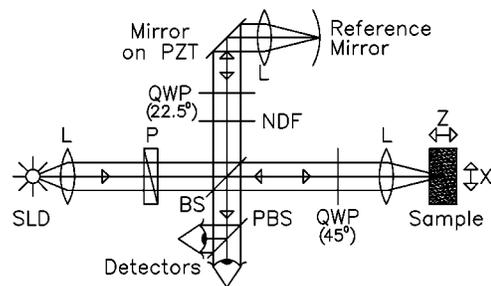
**Fig. 1** Schematic of the PS-OCT device. SLD, superluminescent diode; L, lens; P, polarizer; BS, beamsplitter; QWP, quarter-wave plate; NDF, neutral-density filter; PBS, polarizing beamsplitter; PZT, piezoelectric transducer. Two-dimensional images were formed by lateral movement of the sample at constant velocity (x direction), repeated after each axial displacement (z direction).
