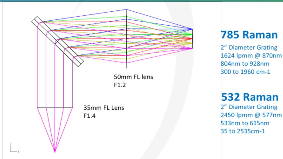
Figure 4 –Diagram of two different Raman sources with different gratings
