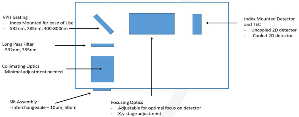
Figure 3 – Block Diagram of the Internal Components, with some having multiple options
