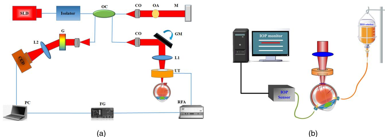
**Fig. 1** (a) Optoacoustic elastography setup with unscalded porcine eye. SLD, superluminescent diode; OC, optical coupler; CO, collimator; OA, optical attenuator; M, mirror; GM, galvanometer mirrors; L1/L2: lens; UT, ultrasonic transducer; RFA, radiofrequency amplifier; FG, function generator; and G, grating. (b) Schematic of the IOP control and measurement system.
