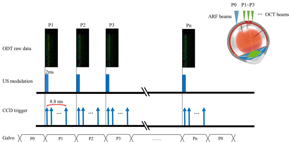
**Fig. 2** Schematic representation for synchronization of the complete imaging system for synchronized confocal OCE. M-mode displacement map data were acquired in each location (e.g., P0, P1, P2, etc.).
